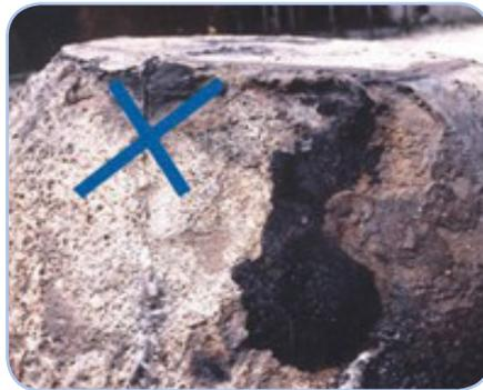
Figure 4. Flame directed to one spot on a crucible produced this damage.
