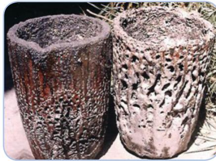
Figure 8. Overfilling caused flux to chemically attack the exterior of these crucibles.
