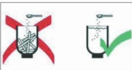
Only add flux after the metal is molten.
