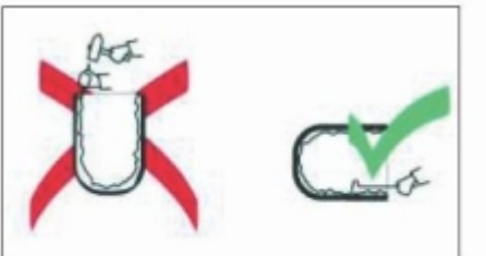
The crucible should be cleaned out carefully every day while still red hot.
