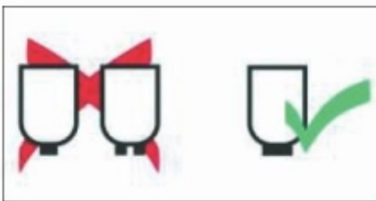
Use the correct crucible stand which must be central and support the whole base.
