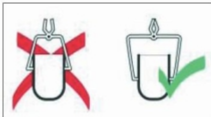
Lift-out tongs should hold crucible on its lower third and fit evenly on both sides.
