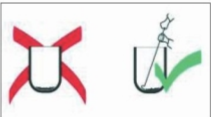
The crucible must be emptied before switching off the furnace.
