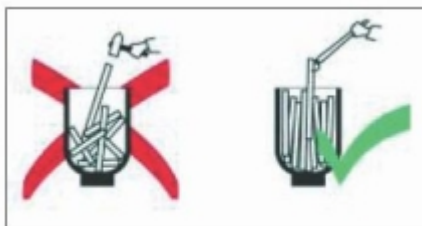
First charge with light returns, as a cushion, then add ingots vertically.
