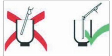
Ingots should be loaded carefully into the crucible using tongs.
