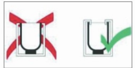
Allow space for expansion between crucible and furnace lining/cover.
