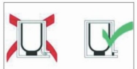
Avoid ingress of cold air by ensuring that the drain hole is sealed.
