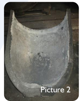
Picture 2 TBNS 587 Z2e 2 PRO Coating after 220 batches.
