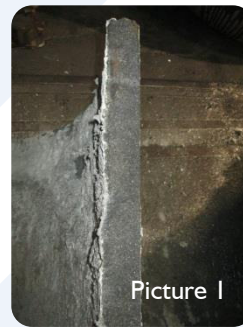
Picture 1 TBNS 587 Z2e 2 PRO Coating after 220 batches.
