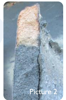
Picture 2 Syncarb Z2e 2 brim oxidation after 12 months.
